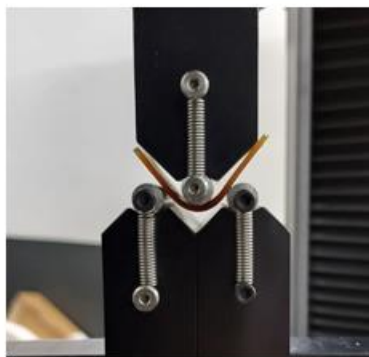
Figure 4.9. Flexural test for BIO-PUR1.
