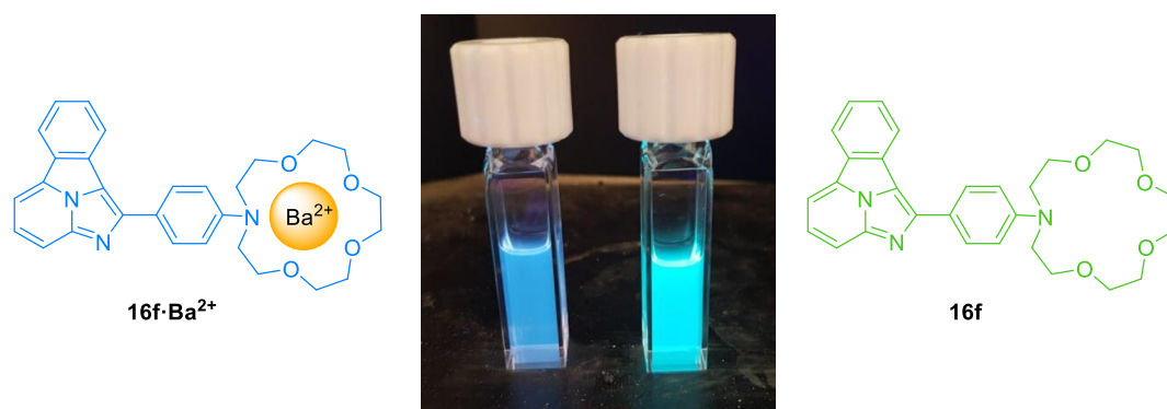
Figure 42.- Photograph and structures of 16f and 16f·Ba 2+ in acetonitrile showing bicolor emission upon irradiation at 365 nm.
