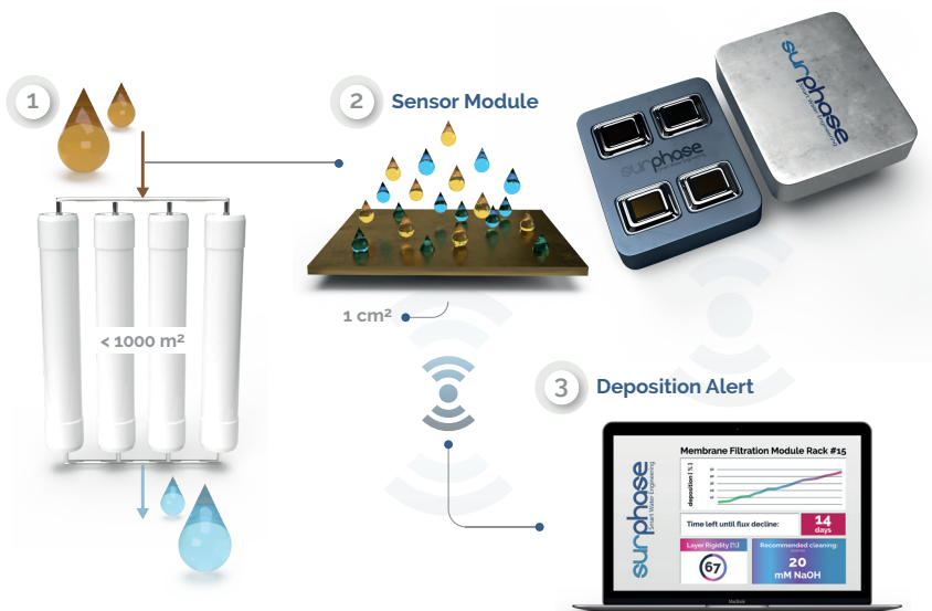
Figure 7.4. Schematic of the installation and concept of the fouling monitoring device. 1: RO unit; 2: monitoring sensorial device (schematic); 3: software for data acquisition and visualization.
