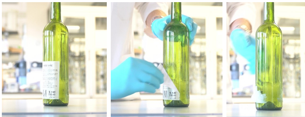
Figure II.6. Paper label attached to a glass bottle with PSA which includes a synthesized oligoester crosslinker (ASY-LA8CL4) after immersion into a basic aqueous solution for 24 h.
