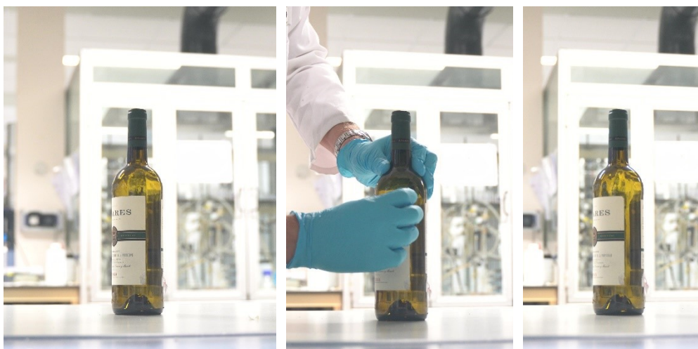
Figure II.5. Commercial wine bottle with commercial label and PSA after immersion into basic aqueous solution for 24 h.
