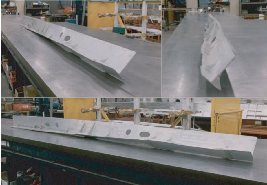
FIGURE 2.6: Distortion due to stress relaxation of a C-17 Cargo floor beam machined from die forging, with no stress relief [22].
