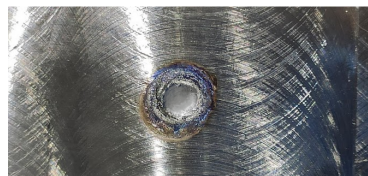
FIGURE 4.20: Footprint after electropolishing at 0.12 mm depth after four iterations.
