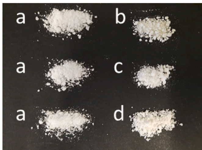
Fig. 10. Color evolution of the samples after the thermal endurance test (solid state): a) fresh xylitol; b) xylitol maintained at 100 °C during 150 days; c) xylitol maintained at 120 °C during 30 days and d) xylitol maintained at 175 °C during 72 h.
