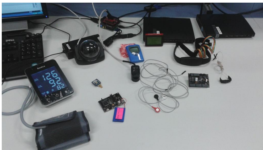
Figure 12. Infrastructure of the healthcare demonstrator: e -Health Sensor Platform V2.0., gas sensors kit and processing units.
