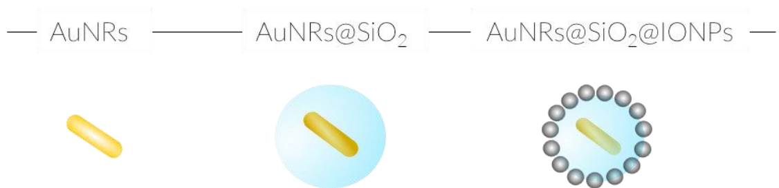
Figure 4.1. Schematic representation of the NPs obtained at each synthetic step. In this process, AuNRs were synthesized, covered by mesoporous silica (AuNR@SiO 2 ) and IONPs were finally grown onto the silica shell to obtain AuNR@SiO 2 @IONPs.
