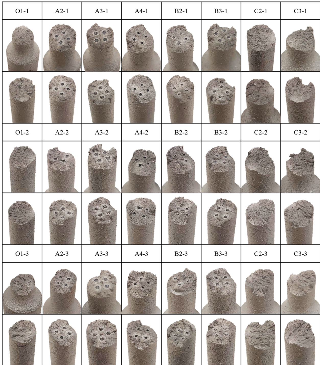
Fig. 1 – Fracture image of each AlSi10Mg specimen.
