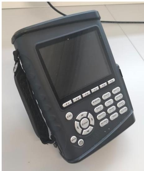
Figura 109. Transductor CoCo 80.
