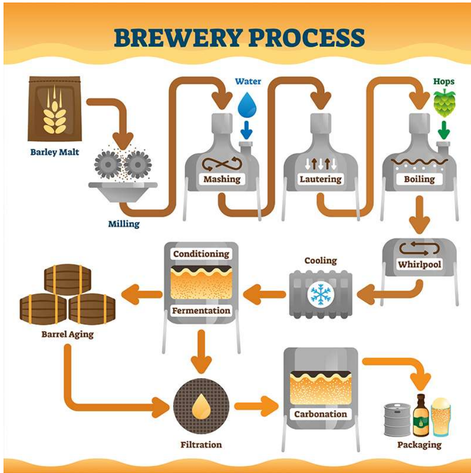
Figure 1: Brewing process diagram (Cocinista, 2010)
