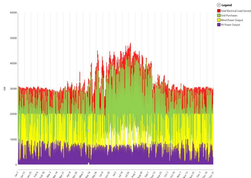
Figure 43. Generation and Consumption in a Hybrid System with the grid and a high alternative of PV and Wind Power.
