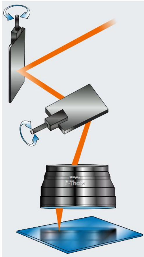
Figure 8 The galvanometric mirrors and the F-Theta lens [13]
