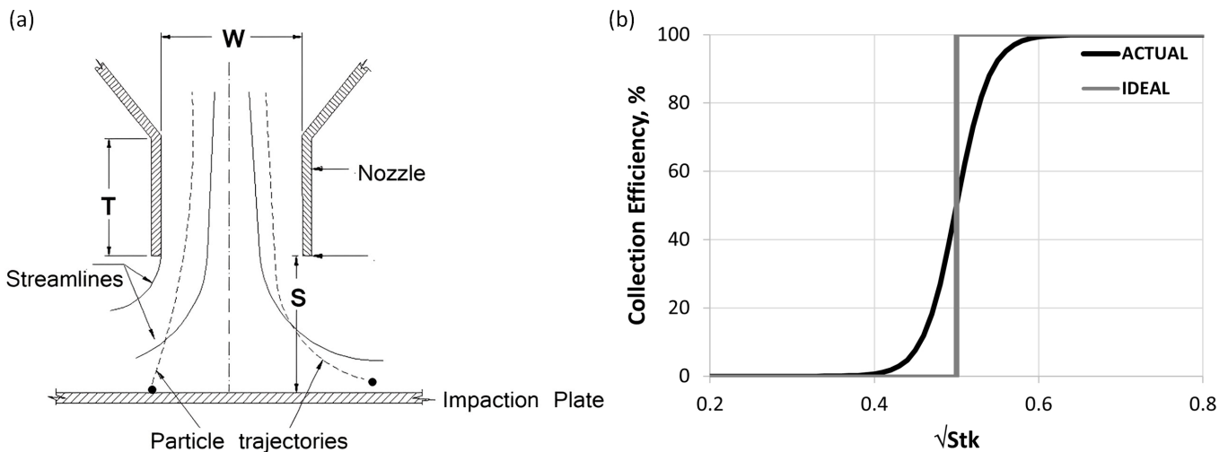
Fig. 1. (a) Single nozzle inertial impactor; (b) Ideal and actual collection efficiency curve as a function of Stokes number (i.e., \sqrt{Stk} ).
