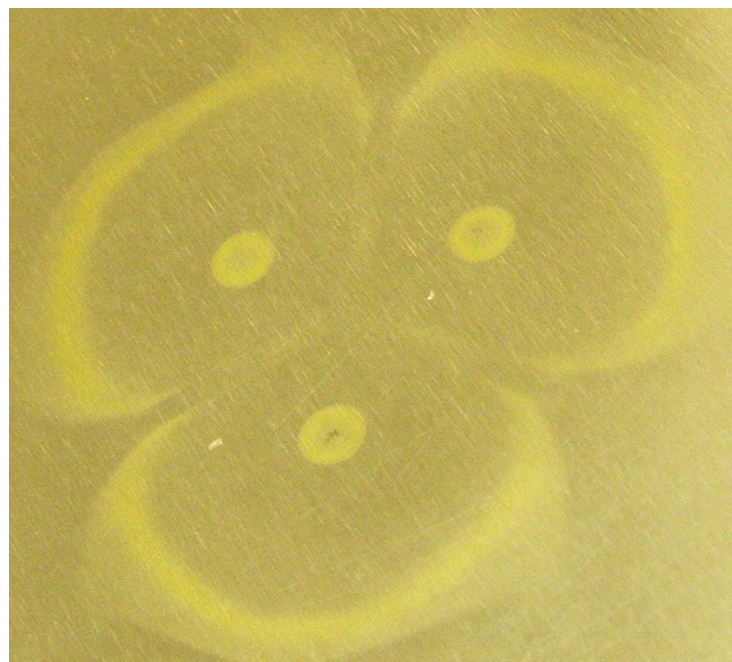
Fig. 5. Halo formation on impaction plate for 3-nozzle impactor at A/W = 6 and Re = 1380 (García-Ruiz et al. , 2019a).
