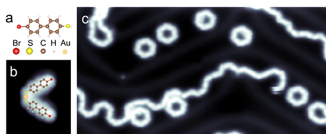
Figure 1. Thioether structures formed on Au(111) surface. a. Sketched molecular structure. b. Topographic image of a Br-MBP dimer ( 3 \times 3.5 \text{ nm}^2 ), c. Topographic image of the polymer structures formed after the annealing of 4'-Bromo-4-mercaptobiphenyl (Br-MBP) molecules ( 30 \times 15 \text{ nm}^2 ; 1 V, 0.3 nA).
