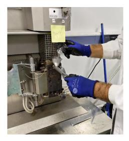
Figure 5 : PLLA injection in the DSM
