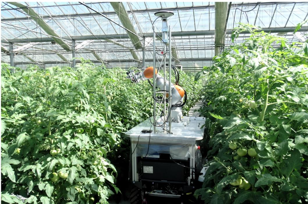
**Fig. 4.8.** – The platform inspecting plants while navigating through the greenhouse. Note the difference of the plants at the beginning of the development (top) compared to some months later (bottom). In that period, the platform was modified and *grew* as well.
