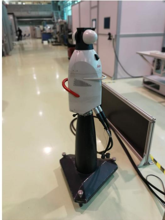
Fig. 3.1. – The laser tracker used to measure distances with a micrometric accuracy. It serves as ground truth to measure localisation errors.
