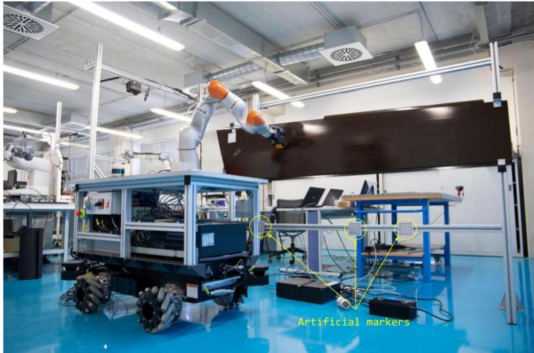
Fig. 4.3. – The accurate positioning and inspection scenario. The platform is positioned in front of the first label, and the arm is performing the inspection of the first part. Under the aileron, the label for the next scanning position can be seen.
