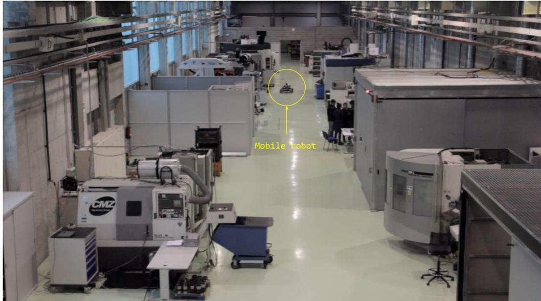
Fig. 3.2. – West half of the workshop. At the top, the mobile platform navigating.
