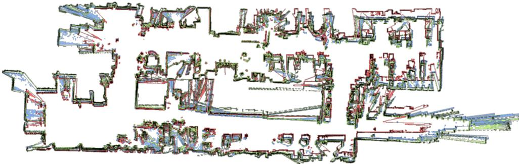
Fig. 3.3. – Overlapping of the maps obtained with each algorithm: *gmapping*, blue; *hector\_slam*, red; *cartographer*, green.
