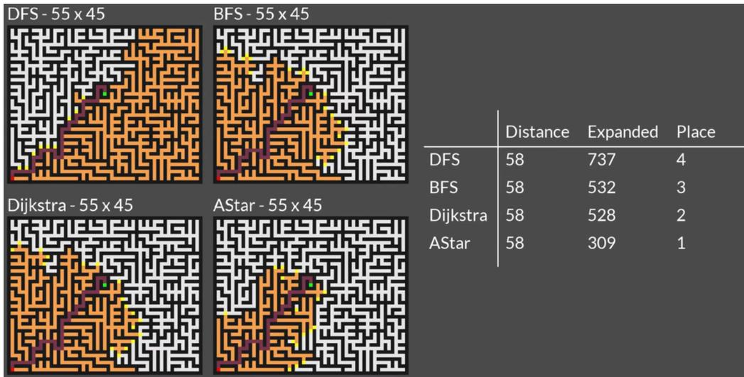
Fig. 2.8. – A comparison of the main path-finding algorithms in a 55x45 cell example maze and a random destination point. White colour depicts the free unexplored space, black are the obstacles (or walls), green is the destination point, red the origin (or robot position), orange colour represents the explored nodes, yellow the next nodes to analyse, and maroon is the trajectory found. On the right-hand side of the image, some metrics of their performance are shown [215].
