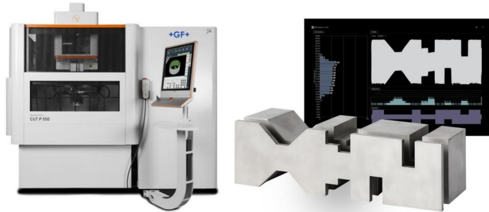
Figure 6. (a) AgieCharmilles CUT P 550 WEDM machine; (b) Result of spark tracking [16].
