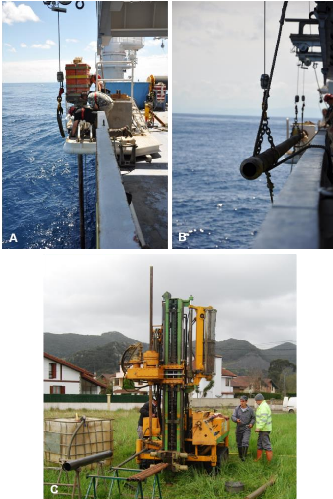
Figure M.3 – A and B) Core extraction with a Kullenbeg corer during the EUSKASED (Euska2) campaign on board the R/V Côtes de la Manche cruise ship in 2004. C) Drilling boreholes with ROLATEC RL-46 a percussion/rotary drill in Liendo (Cantabria).
