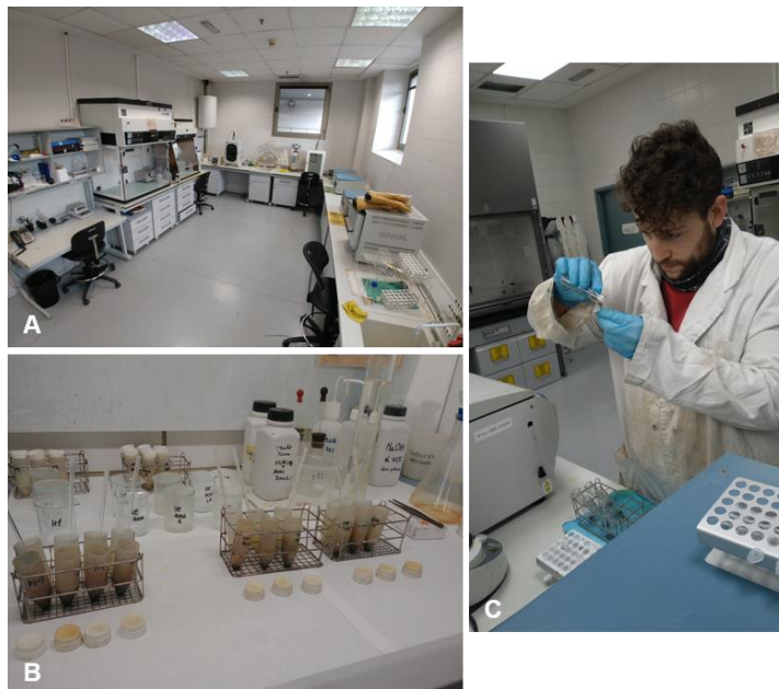
Figure M.6 - A) Laboratory for chemical treatment of pollen samples at CCHS (CSIC) in Madrid. B) Pollen samples prepared for HF treatment. C) Samples stored with glycerine in Eppendorf tubes. Photographs by Reyes Luermo-Lautenschlaeger.
