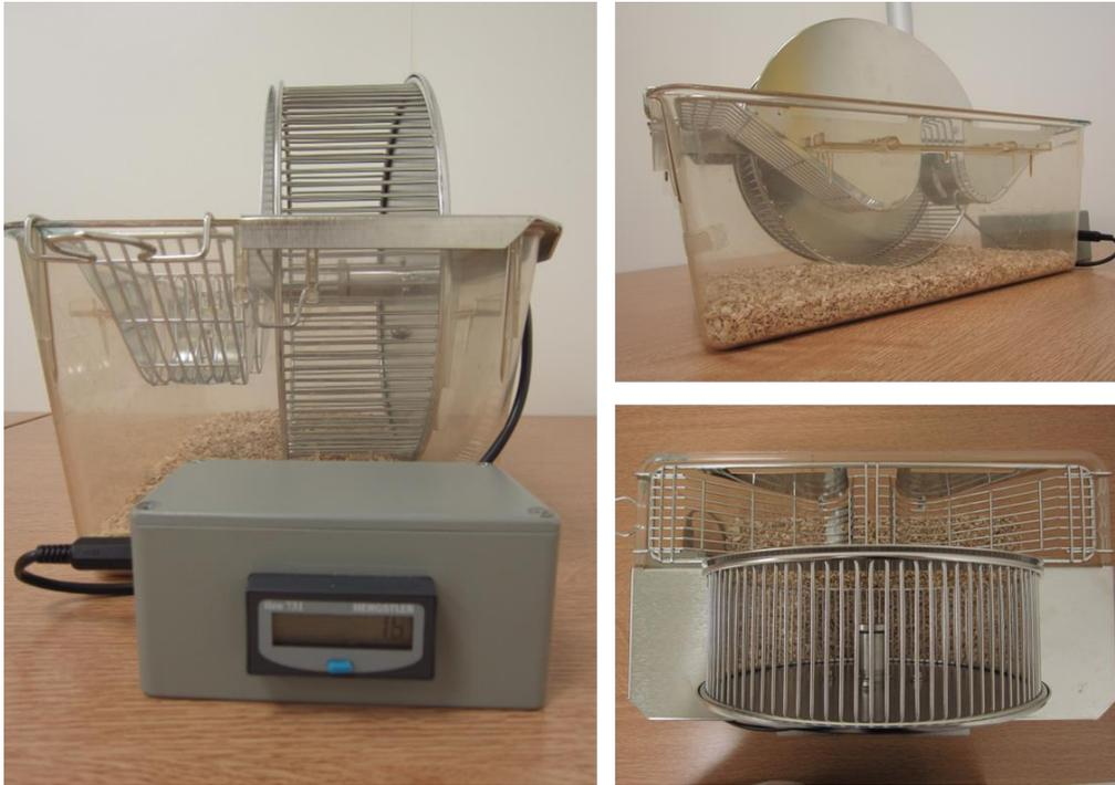
**Figure 7.** Activity wheel adapted for mouse cages used in the experiments performed in this doctoral thesis. Activity wheels were introduced in the cages inside the hypoxia chamber, working at low concentration levels (10%) or room air.
