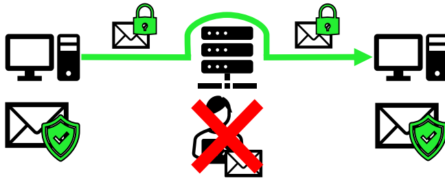
Fig. 2.3 Application layer E2E security. Middleboxes only have access to the information they need to forward the message to the next endpoint.
