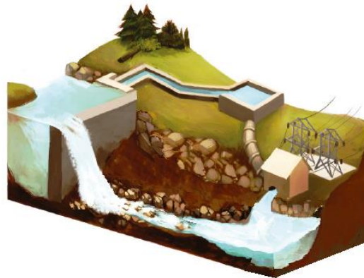
Figure 4. Schematic picture of a diversion run-of-river scheme. Modified from Couto & Olden, 2018.
