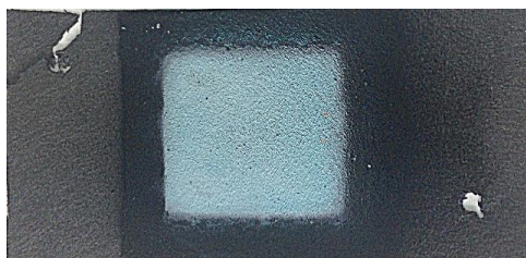
Figure 3.6. Appearance of MOF-GDE of 10 \text{ cm}^2 obtained after airbrushing catalytic ink keeping 1 \text{ mg}\cdot\text{cm}^{-2} of loading.
