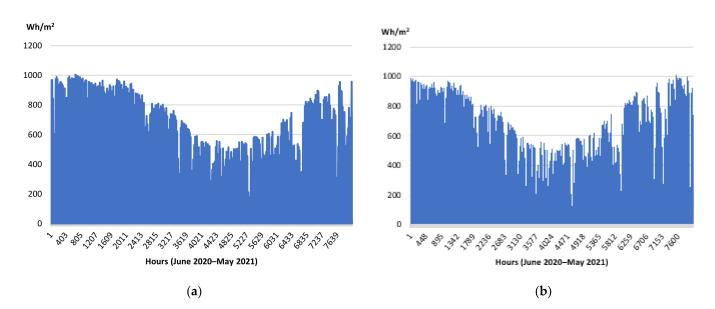
Figure 6. Hourly Wh/m<sup>2</sup> irradiation for a year: (a) Tolosa and (b) Malaga.
