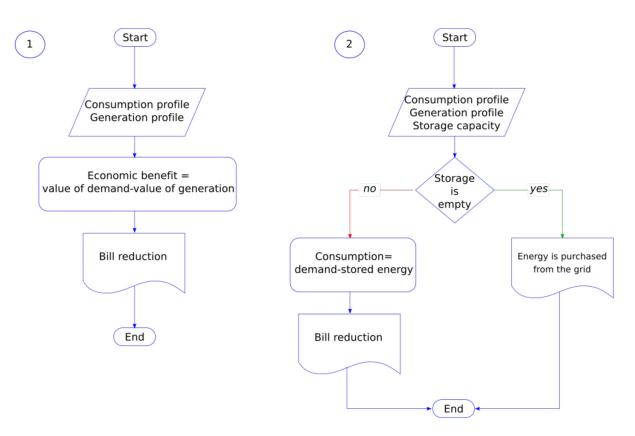
**Figure 5.** Flowcharts for managing a virtual LEC. (1) It is not considered to be a storage system. (2) It is considered to be a storage system.
