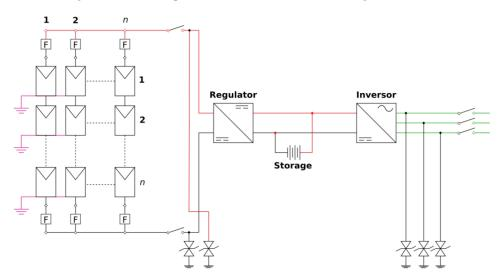
Figure 7. General electrical diagram of the photovoltaic installation.
