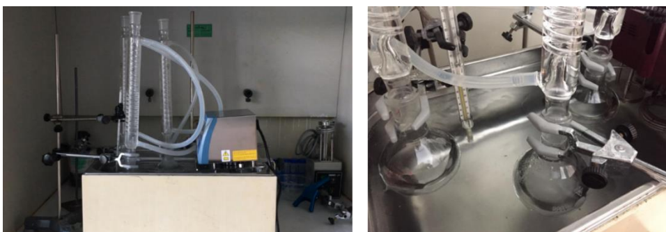
Figure 4.28. One of the experiments batches containing three flasks with three different concentrations, submerged in the water bath at 90 °C.
