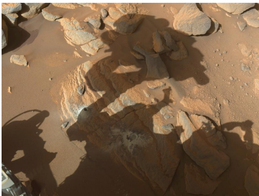
Figure 4.10. NavCam image (left camera) of the workspace showing the Dourbes abraded patch and the Sallette hole remaining after extracting the core to be returned to Earth. Ref. NLF_0262_0690212241_488CWS_N0080000NCAM00705_0A00LLJ01-stretched-v2.
