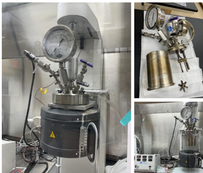
Figure 3.19. Parr 4848B reactor controller
