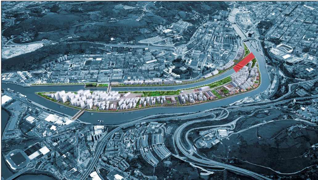
Figure 2: The Zorrotzaurre urban regeneration project is still unfinished. The Deusto Canal was an artificial channel whose use had become obsolete after opening the outer Port of Bilbao in 2006. The opening of the Deusto Canal (red) has converted Zorrotzaurre into an island and has reduced the flooding risk in various neighbouring areas. Source: Zorrotzaurre Management Commission ( http://www.zorrotzaurre.com/ ).
