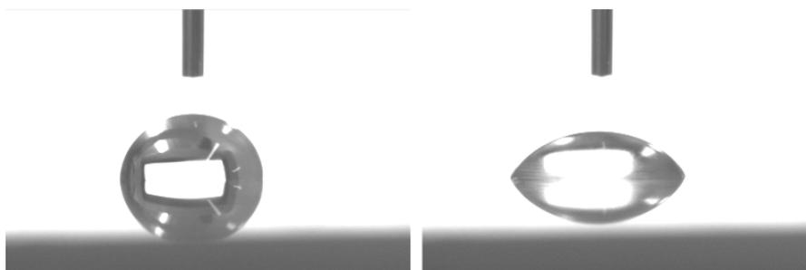
**Figure 1.** Ultrasonic expansion of a 5  $\mu\text{L}$  water droplet [19]. The left image shows the initial state of the droplet. The right image shows its expansion after ultrasonic vibration is applied at 20 kHz.
