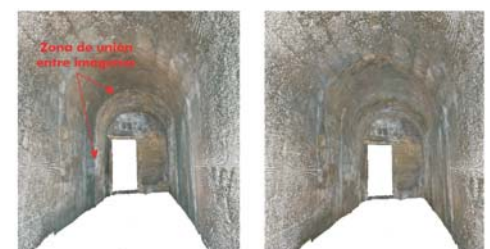
fig 6.- Point cloud before (left) and after (right) the radiometric balance with gradient.
