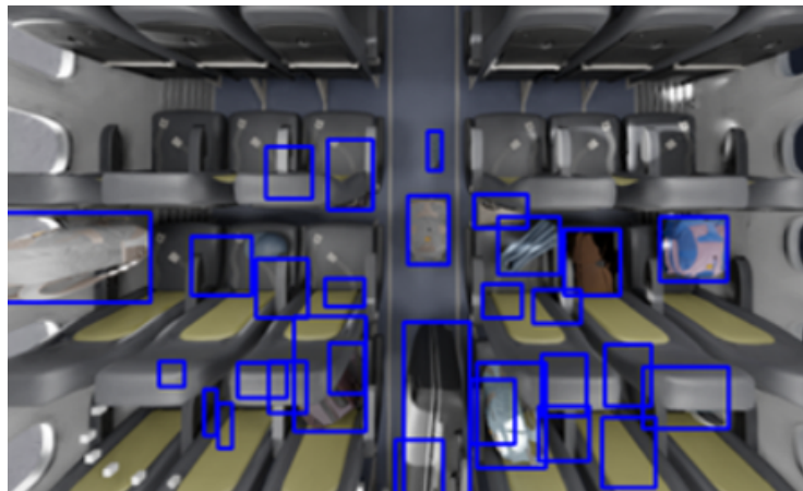
Figure 5.3: Object annotations based on 3D coordinates can result in some annotated objects occluded by the seats.
