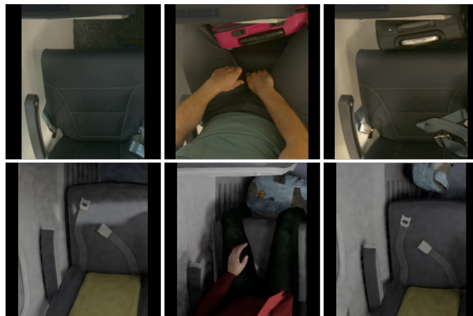
Figure 5.9: Real (top) and synthetic (bottom) ROI samples for training a classification DNN with correct and incorrect situations.
