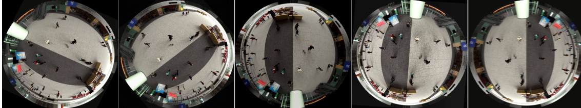
Figure 4.7: Image augmentations applied to a rendered image sample. Color space augmentations are combined with geometrical transformations to generate new augmented samples.
