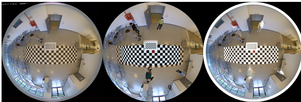
Figure 4.2: a) Image of a real scene; b) The same scene virtually rendered on top of the real image (patterns do not match); c) Virtual and real patterns match after the rectification step.
