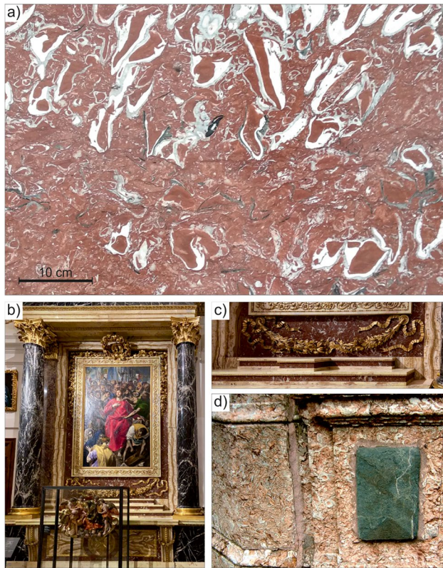
Fig. 6 a Recently restored and newly polished covering slab of the Sota building in Bilbao. Longitudinal section of polyconitid rudists. b, c Red Ereño in the Sacristy of Toledo Cathedral (Spain). They are behind the painting “The Despoilment of Christ” by El Greco. The front columns are from the Black Markina ornamental limestone (Bizkaia, Spain). d Column discoloured by differential erosion processes from the rear door of the garden of the Victor Chávarri Palace in Bilbao (Basque Country, Spain)
