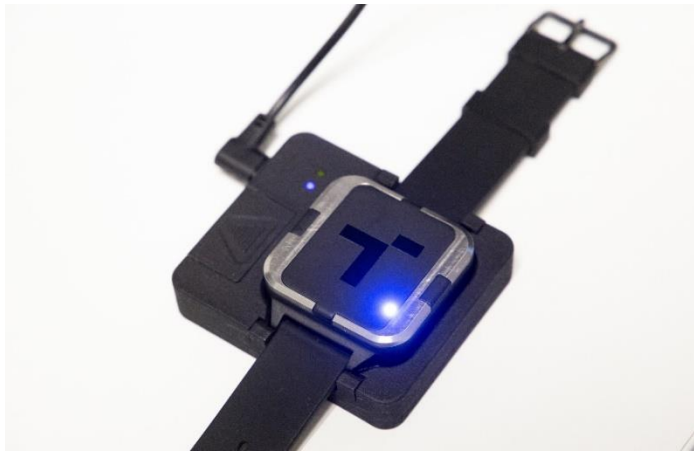
Figure 6.1-8: Wristband on the charging station.
