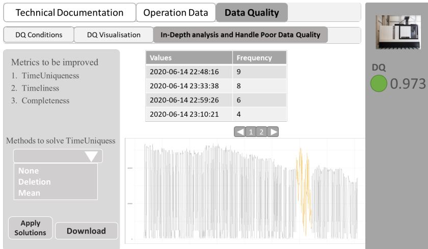
Fig. 2.4.: Example of integration of the dqts package in an industrial system for the evaluation and correction of manufacturing data.
