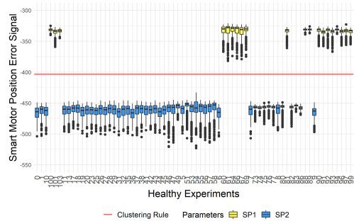
Figure 3. Boxplots of healthy tests, red line represents the operation configuration decision rule.
