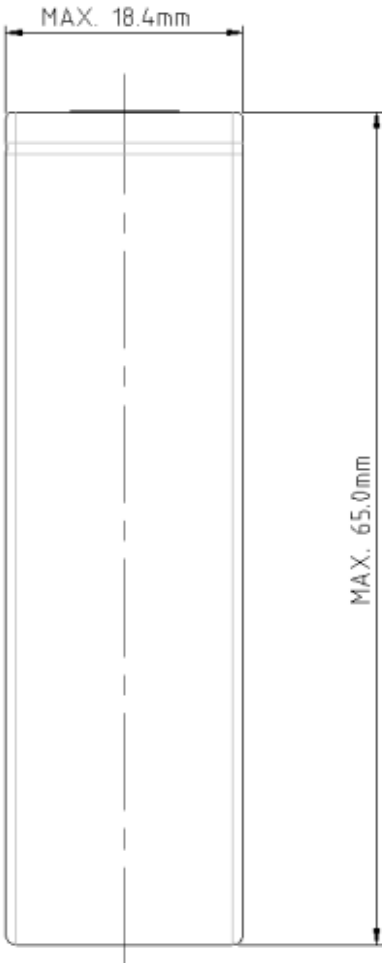
Fig.1. Outline Dimensions of ICR18650-26F
