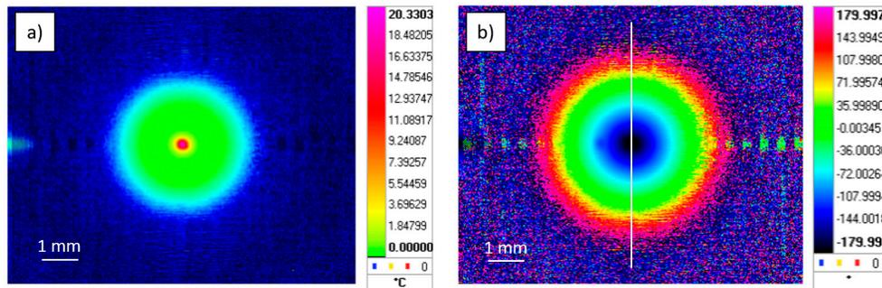
**Figure 5.** (a) Amplitude and (b) phase thermograms of Sample 1 at the surface 0 mm from the substrate, with a modulation frequency of 7 Hz. The white vertical line corresponds to the phase profile used for thermal diffusivity measurements. The scale of the amplitude is in  $^{\circ}\text{C}$  and the phase is in degrees.
