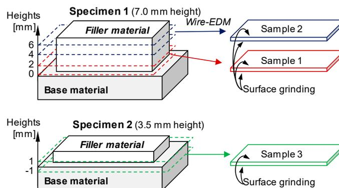
**Figure 2.** Sample extraction for thermal diffusivity measurements.
