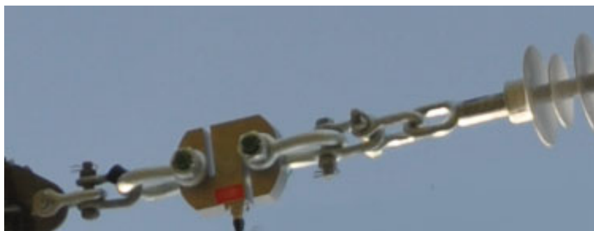
Fig. 2. Load cell for measuring the conductor tension
