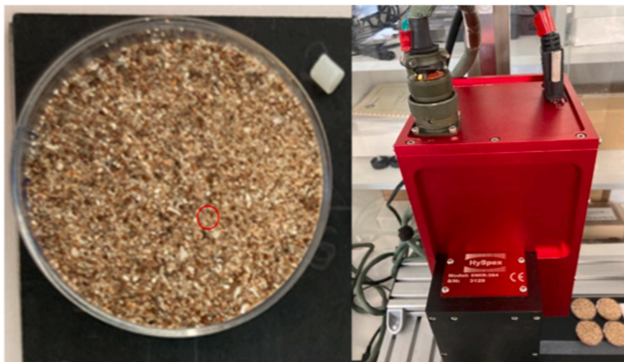
Fig. 2. (Left) Petri dish of sand doped with one ABS MP, circled in red, along with reference plastic pellet (white pellet on the top). (Right) NIR-HSI hyper-spectral camera.
