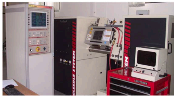
Fig. 2. Thermomechanical test set-up for hot compression tests.
