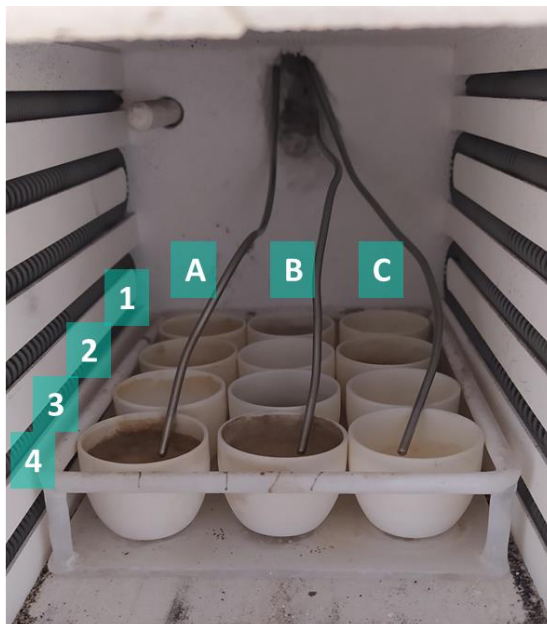
Figure 11: Photography of the 12 crucibles placed in the quartz tray inside of the oven. The thermocouples used for the oven calibrations can be observed inside of three of the positions. The labelling of the crucibles is also indicated by a combination of columns (A, B and C) and lines (1, 2, 3, 4).
