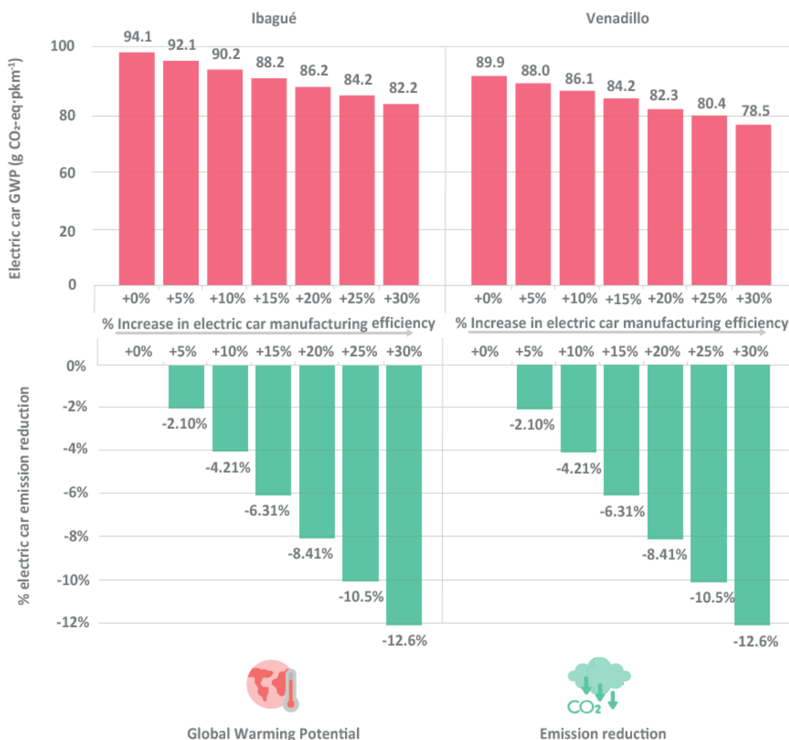
Figure 7. Sensitivity analysis of EV Global Warming Potential with increases in EV manufacturing efficiency.
