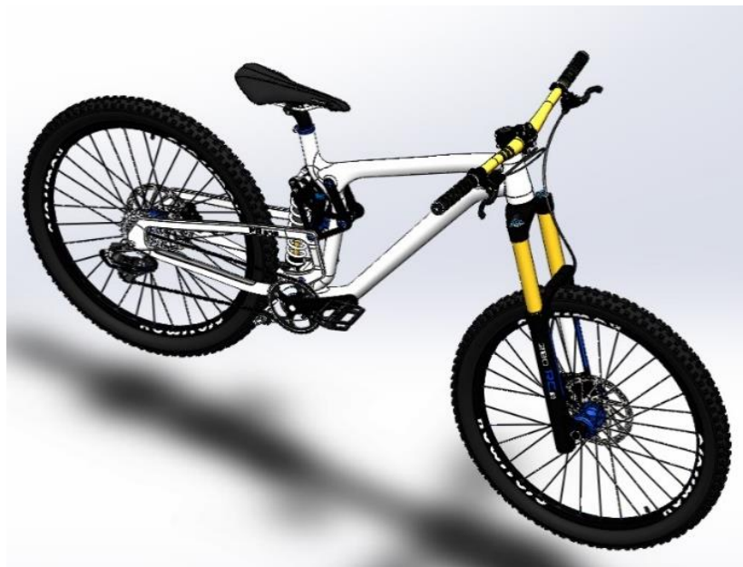
Figure 24. Design of the selected bicycle modelled in SolidWorks.
