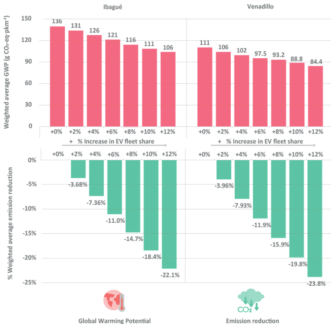
Figure 8. Sensitivity analysis of average GWP with increases in the fleet size of electric vehicles.
