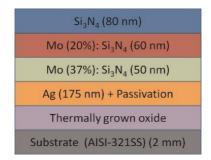
Fig. 1. Schematic representation of the solar selective coating.
