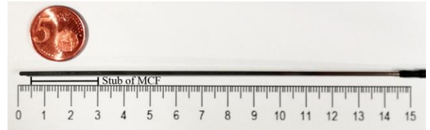
Fig. 4. Picture of the manufactured MCF sensor after being exposed to 1000^\circ\text{C} . Notice that the metallic tube has a blackening gradient that indicates the different temperatures on the tube. The position and length (2.54 cm) of the MCF segment are indicated. The gap between the tip of the metallic tube and the stub of MCF is long enough to avoid a Fabry-Perot cavity.
