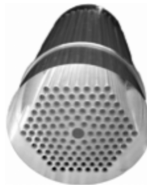
Fig. 1. Digital camera photograph of the drilled preform with a diameter of 60 mm.
