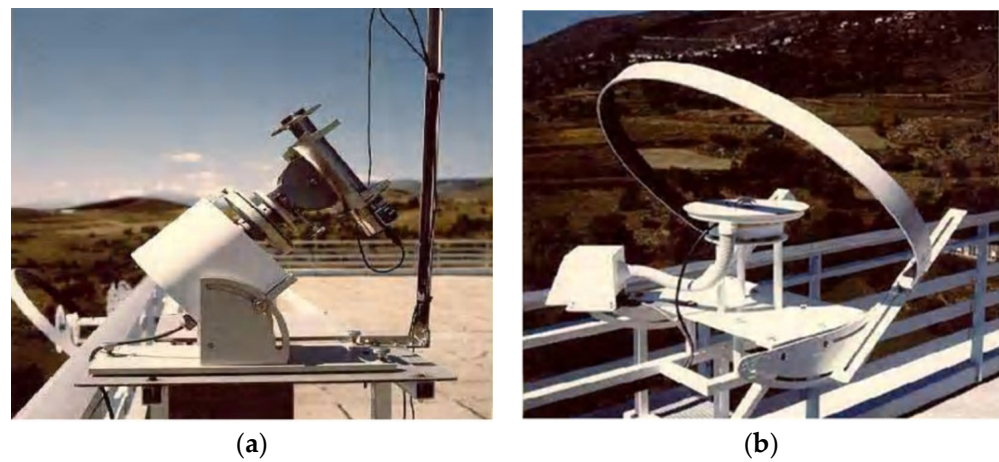
Figure 4. Instruments for measuring solar radiation: (a) pyrheliometer; (b) pyranometer.
