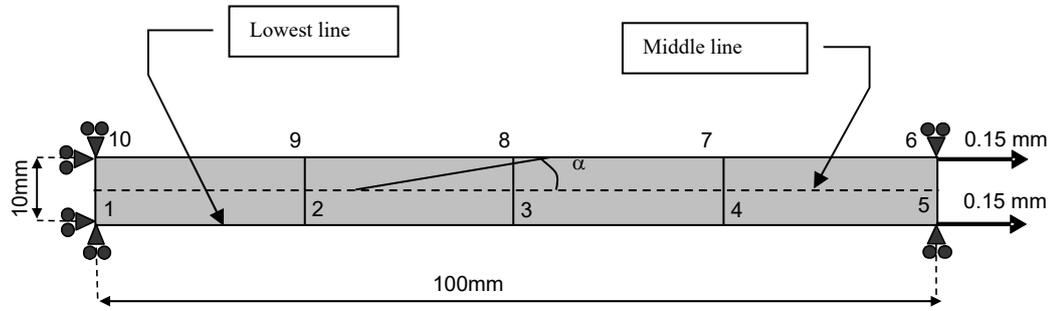
Figure 7. Displacements in the off-axis tensile specimen:
