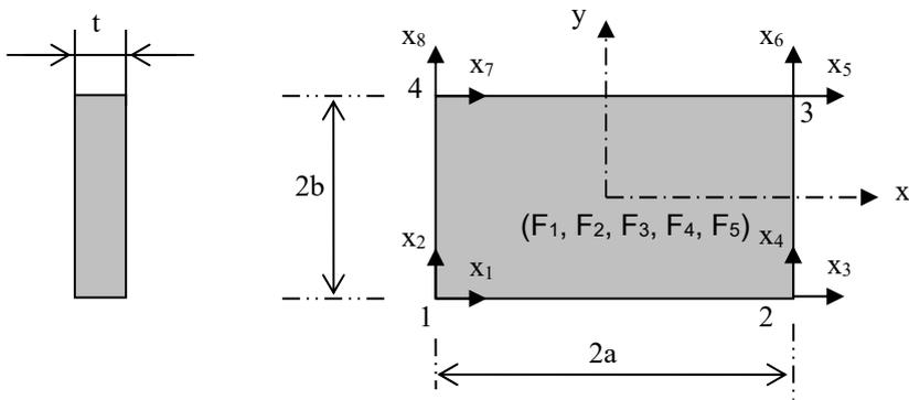
Figure 2. Cantilever beam with two tip forces at the end.
