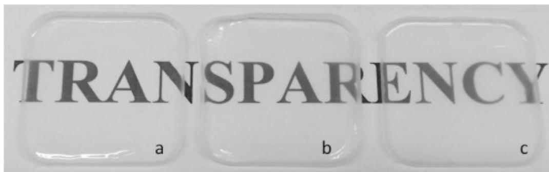
Fig. 2. (a) WBPU matrix, (b) WBPU-1<sub>son</sub> and (c) WBPU-1<sub>syn</sub> nanocomposites films prepared by casting.
