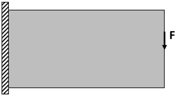
Fig. 12 Design domain of a cantilever beam
