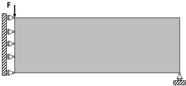
Fig. 7 Design domain of a half MBB beam
