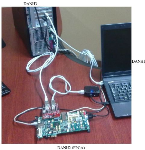
Figure 13. HSR ring implemented using 2 PCs and an FPGA running the HSR software.
