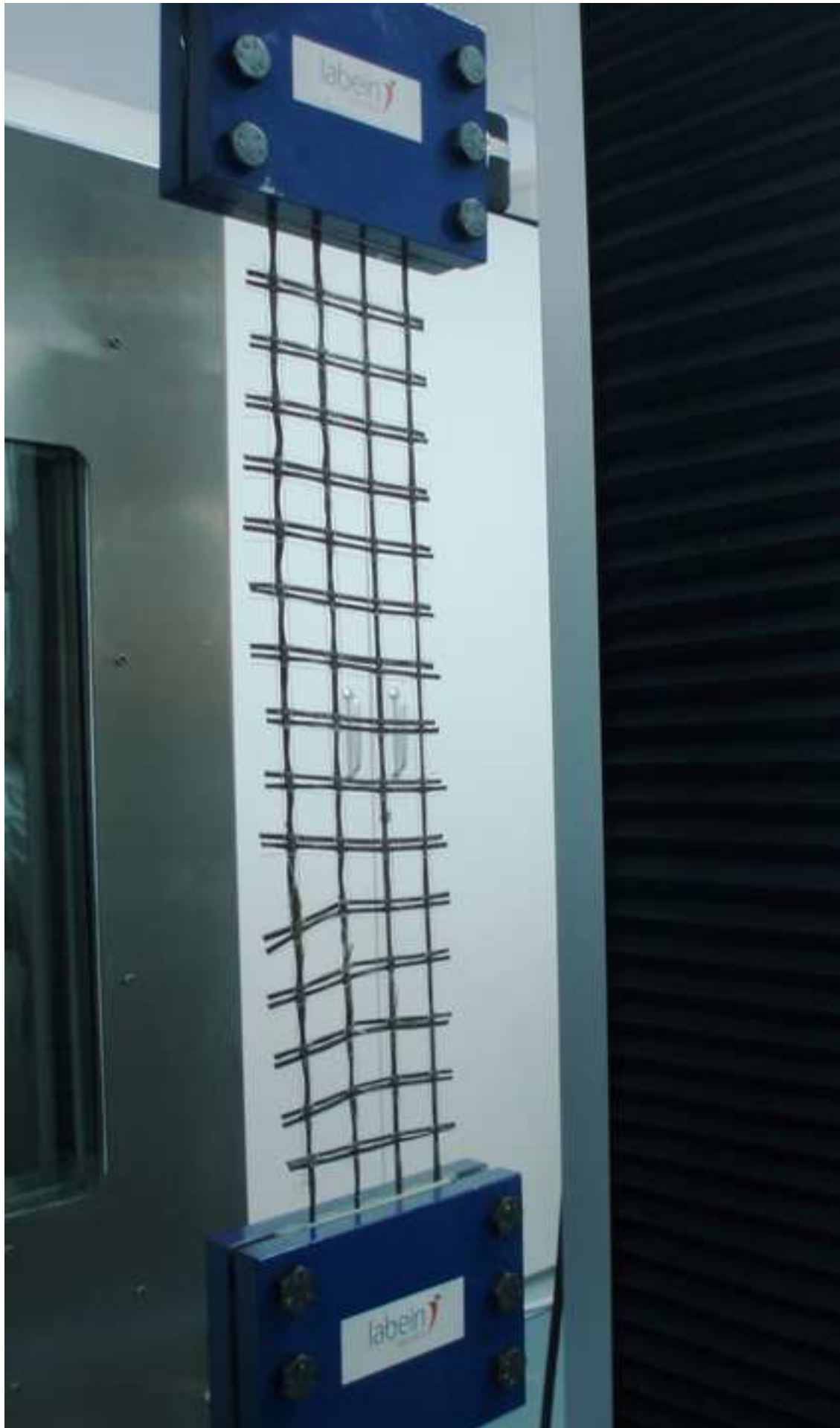
Figure 2. Pure tensile tests of several basalt textile specimens Click here to download high resolution image
