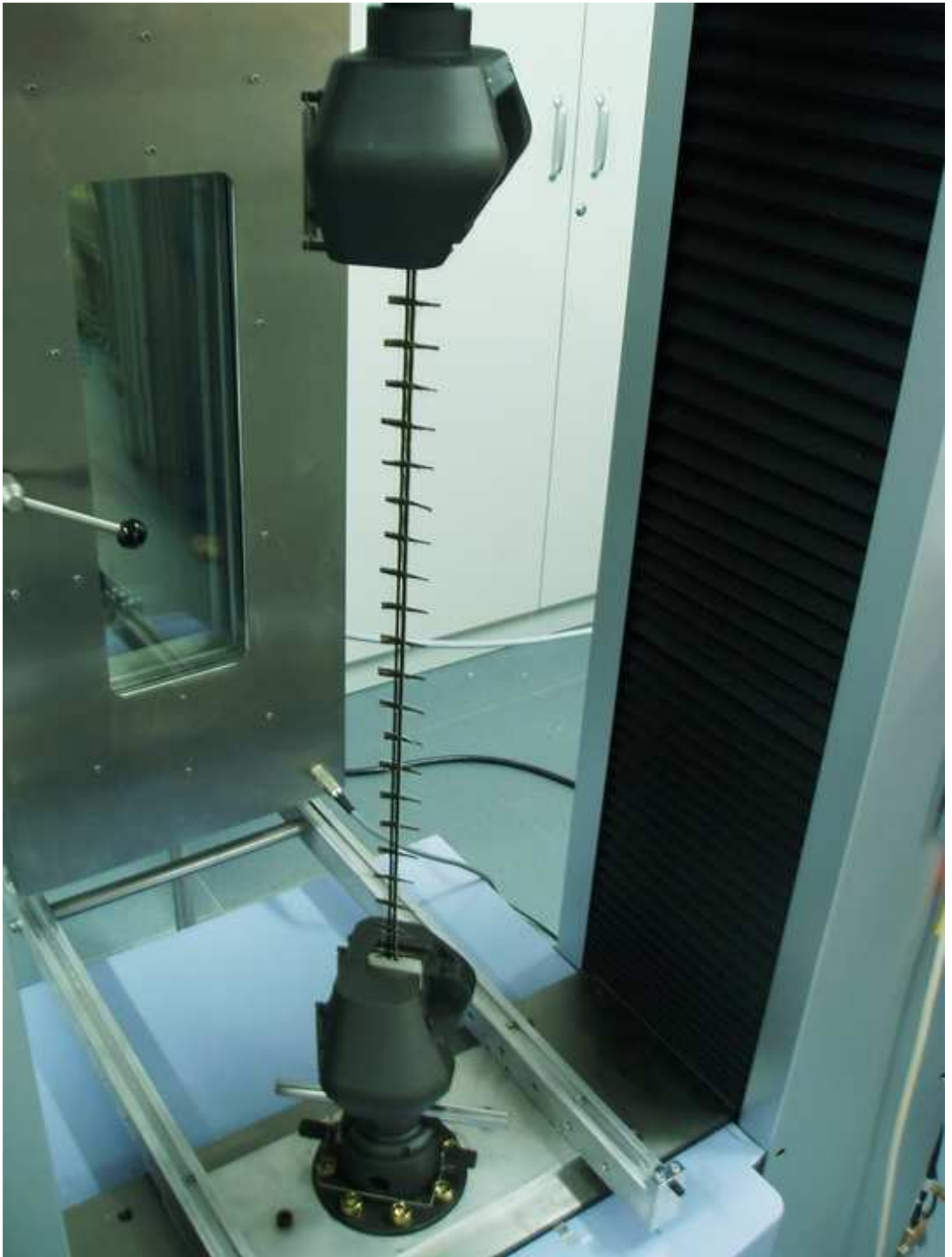
Figure 2. Pure tensile tests of several basalt textile specimens Click here to download high resolution image
