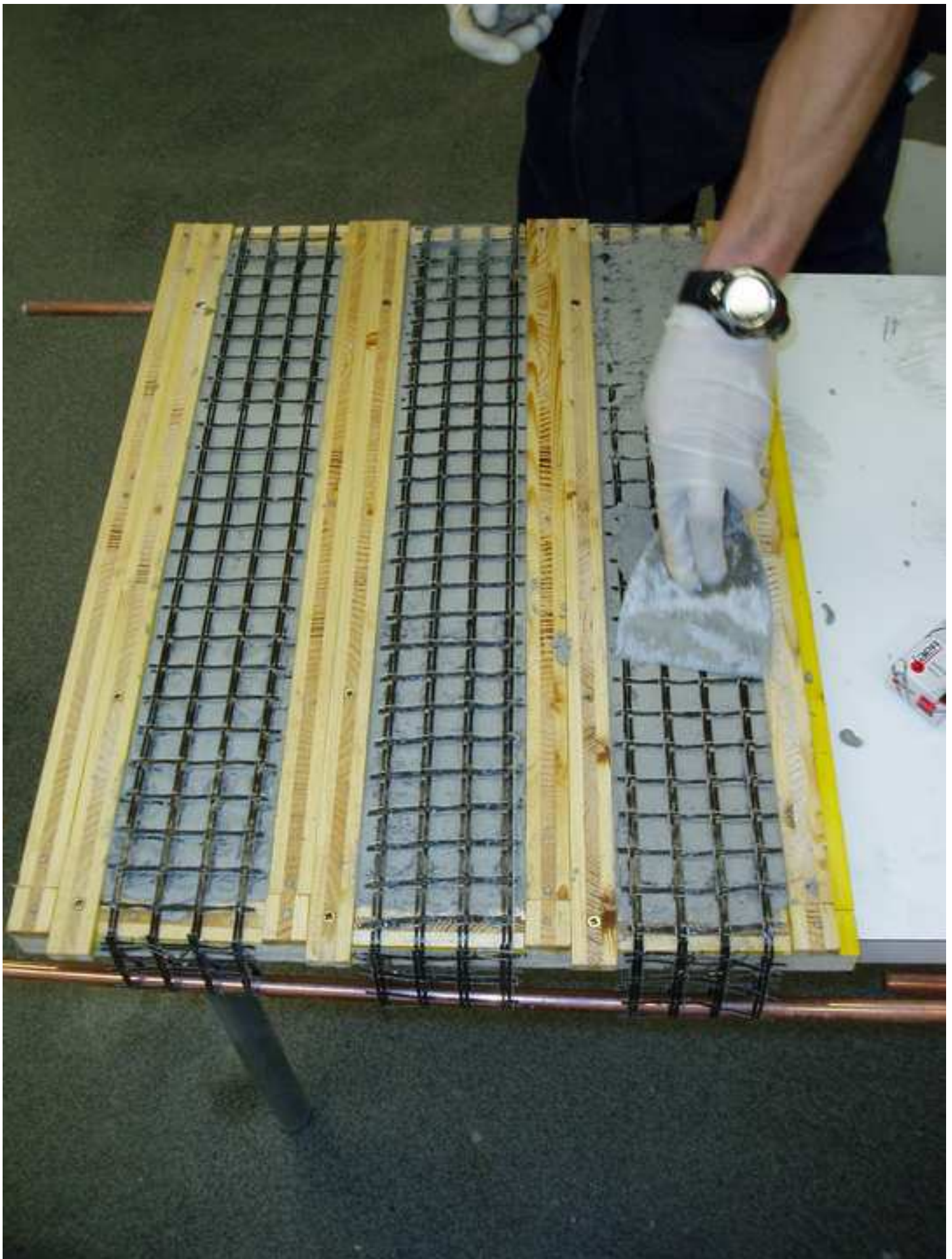
Figure 3. Preparation and testing of the TRM specimens Click here to download high resolution image
