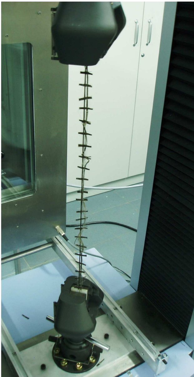
Pure tensile tests of basalt textile specimens 70x135mm (300 x 300 DPI)
