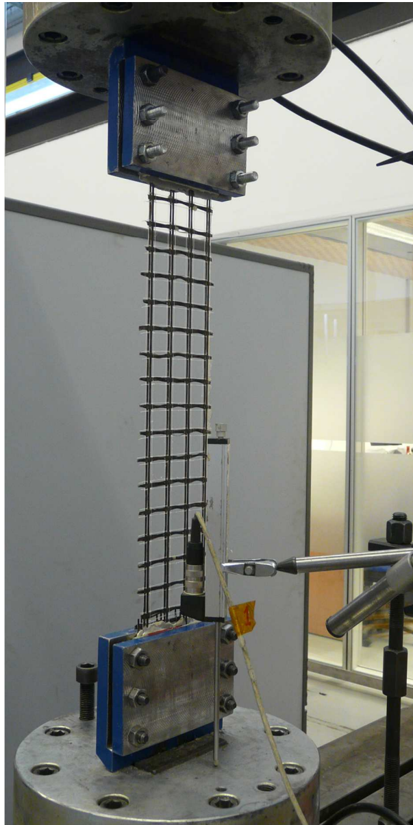
Test set up for pure tensile test of BTRM specimen 70x139mm (300 x 300 DPI)
