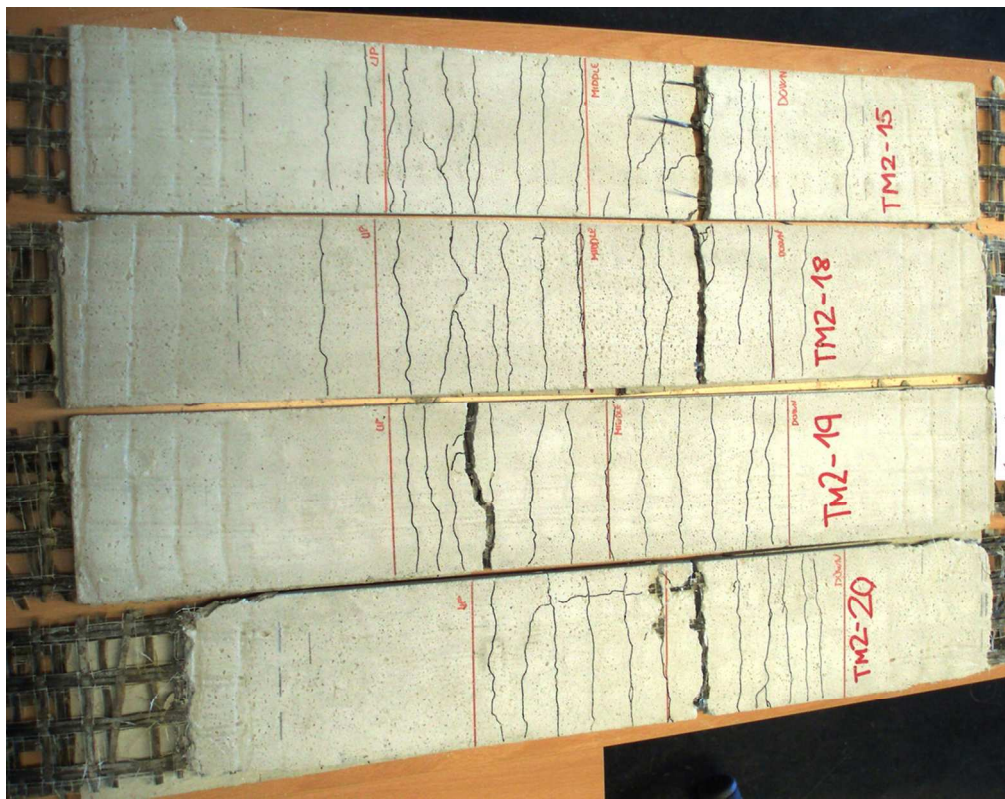
Cracks formed during pure tensile tests of BTRM of M1 (left) and M2 (right) specimens 99x79mm (300 x 300 DPI)
