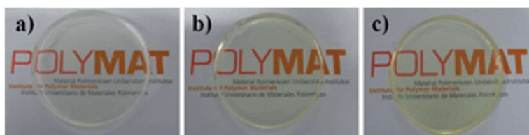
Fig. 12 Photographs of films casted for (a) Run 1 (no CeO 2 ), (b) Run 2 (0.5 wt% CeO 2 ) and (c) Run 3 (1 wt% CeO 2 ).
